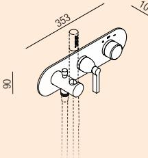
**Built-in thermostatic tap unit with flow deviator and hand-held shower holder /**
