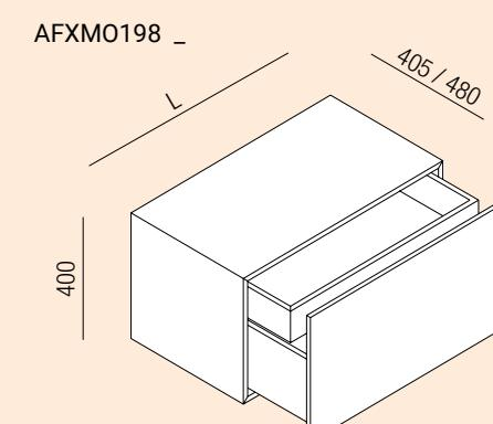
**Storage unit with drawer and internal drawer / Contenitore con cassetto e cassetto interno****L 60 / 80 / 100 / 120 (p. 480) – L 80 (p. 405)**
