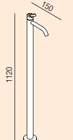
Floor standing washbasin mixer tap with floor connections / Miscelatore lavabo con attacchi a pavimento
