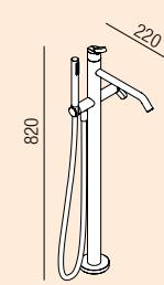
Floor standing bathtub mixer tap with floor connections / Miscelatore per vasca con attacchi a pavimento
