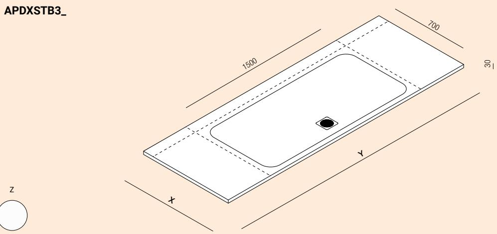
**Custom built shower tray in Ceramilux® with central drain and rectangular basin** / Piatto doccia in Ceramilux® a misura con scarico centrale e invaso rettangolare
