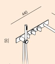
Thermostatic unit for bathtub with hand-held shower, with floor connections / Miscelatore per vasca con doccetta, con attacchi a pavimento
