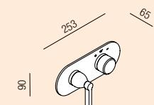
**Built-in thermostatic set with flow regulation with single output /**
